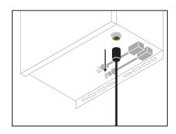
**Step 2** Align notches and plug the cable end into the yellow input on the bottom of the power converter. Gently hand tighten to screw the silver collar into the input.
