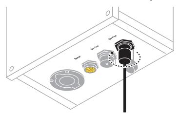
**Warning:** Do not use tools to tighten cap. Cap should be snug, but will not be flush against control box.
