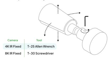
**Step 2** Fully tighten screw on camera neck using provided tool when desired angle is chosen.
