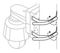
**Step 3** Trim steel straps to desired length using tin snips (not included).
