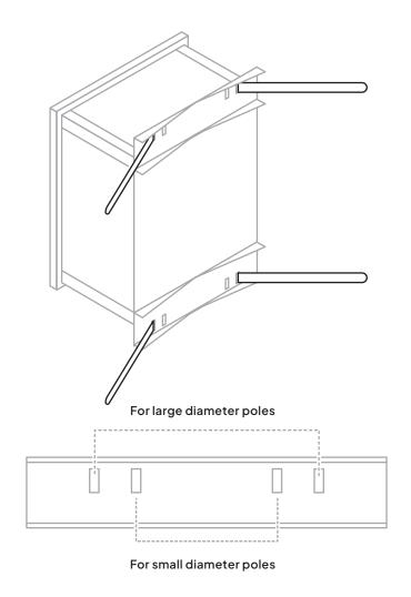
**Step 2** Tighten each strap around pole using drill with 5/16 hex head driver bit.
