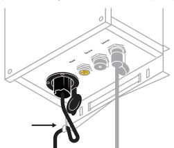
**Step 3** Plug other side of cable into a 110V power outlet.
