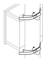
**Step 3** Trim steel straps to desired length using tin snips.
