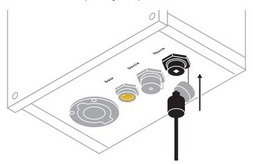
**Step 3** Hand tighten protective cap on camera connector up into bottom of control box. This will create a watertight seal.
