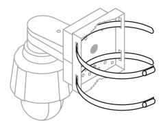
**Step 2** Tighten each strap around pole using drill with 5/16 hex head driver bit (not included).
