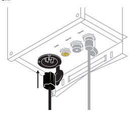
**Step 2** Loop cable onto j-hook to create a drip loop.
