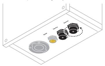
**Step 2** Plug connector coming from camera into input. Connector should snap firmly into place.
