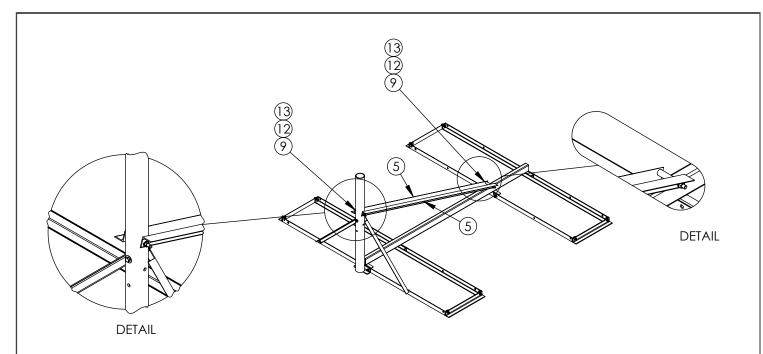
ATTACH THE REAR BRACE(#5) TO THE MAST USING A 3/8"x4" TAPBOLT(#9)FLATWASHER(#12) AND WHIZLOCK NUT(#13). NOTE: THE SLOTTED END ATTACHES AT THE MAST. ATTACH THE OTHER END OF EACH REAR BRACE TO THE SUPPORT TUBE(#2) USING A3/8"x4"TAP BOLT(#9), 3/8" OCKWASHER(#11) & NUT (#10)
