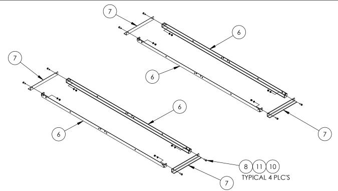
ASSEMBLE THE TWO BALLAST TRAYS (AS SHOWN ABOVE). EACH BALLAST TRAY CONSISTS OF TWO 6' BALLAST ANGLES (#6) AND TWO SIDE PADS (#7). ASSEMBLE EACH TRAY USING FOUR 3/8"x1" BOLTS (#8), NUTS (#10) AND LOCKWASHERS (#11)
