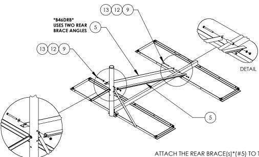
ATTACH THE REAR BRACE(s)\*(#5) TO THE MAST USING A 3/8"x4" TAP BOLT(#9), FLATWASHER(#12) AND WHIZLOCK NUT(#13). NOTE: THE SLOTTED END ATTACHES AT THE MAST. ATTACH THE OTHER END OF EACH REAR BRACE TO THE SUPPORT TUBE(#2) USING A 3/8"x4" TAP BOLT(#9), 3/8" LOCKWASHER(#11) & NUT (#10)
