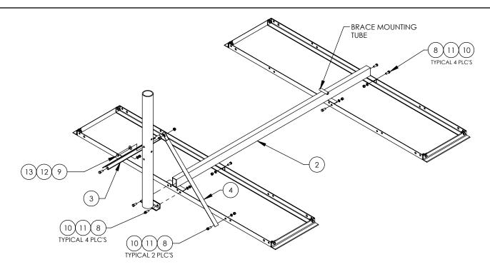
ATTACH THE SUPPORT TUBE(#2) TO THE BALLAST TRAYS USING EIGHT 3/8"x1"BOLTS(#8), NUTS(#10)AND LOCKWASHERS(#11). THE MAST(#1) ALSO GETS ATTACHED AT THIS STEP. ATTACH THE SIDE BRACES (#3 & #4) TO THE MAST USING A 3/8"x4" TAP BOLT(#9), FLATWASHER(#12) AND WHIZLOCK NUT(#13). NOTE: THE SLOTTED END ATTACHES AT THE MAST. ATTACH THE OTHER END OF EACH SIDE BRACE TO THE BALLAST TRAY USING A 3/8" x 1" BOLT(#8), 3/8" LOCKWASHER (#11) & NUT (#10).
