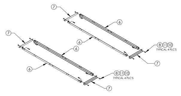
ASSEMBLE THE TWO BALLAST TRAYS (AS SHOWN ABOVE). EACH BALLAST TRAY CONSISTS OF TWO 6' BALLAST ANGLES (#6) AND TWO SIDE PADS (#7). ASSEMBLE EACH TRAY USING FOUR 3/8"x1" BOLTS (#8), NUTS (#10) AND LOCKWASHERS (#11)
