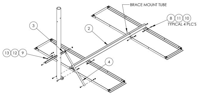
ATTACH THE SUPPORT TUBE(#2) TO THE BALLAST TRAYS USING EIGHT 3/8"x1"BOLTS(#8), NUTS(#10)AND LOCKWASHERS(#11). THE MAST(#1) ALSO GETS ATTACHED AT THIS STEP. ATTACH THE SIDE BRACES (#3 & #4) TO THE MAST USING A 3/8"x4" TAP BOLT(#9), FLATWASHER(#12) AND WHIZLOCK NUT(#13). NOTE: THE SLOTTED END ATTACHES AT THE MAST. ATTACH THE OTHER END OF EACH SIDE BRACE TO THE BALLAST TRAY USING A 3/8" x 1" BOLT(#8), 3/8" LOCKWASHER (#11) & NUT (#10).
