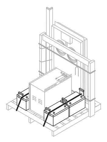
**Step 4** Secure the battery enclosure and batteries with two 145" buckle straps going horizontally across the tops. Thread the straps through the mounting slots on the battery enclosure for extra security.
