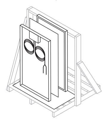
**Step 3** Using the two 115" buckle straps, secure the panels to either side of the upright wooden structure.
