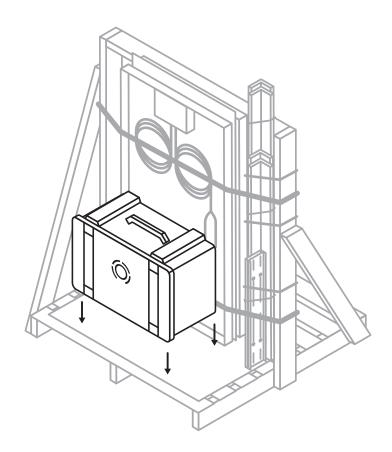
**Step 8** Use one 140" buckle strap to secure the hard case to the upright wooden structure and the other 140" buckle strap to secure the hard case to the bottom of the pallet.
