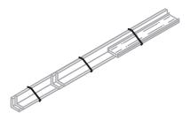
**Step 6** Attach brackets to the upright wooden structure with zip ties. Ensure they're secured on the side with the cardboard so they don't slip through the pallet.
