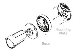
Attach mounting plate to wall or other flat surface, reattach base, then secure camera to base. We strongly recommend that only hand tools, no power tools, be used when mounting or adjusting camera.
